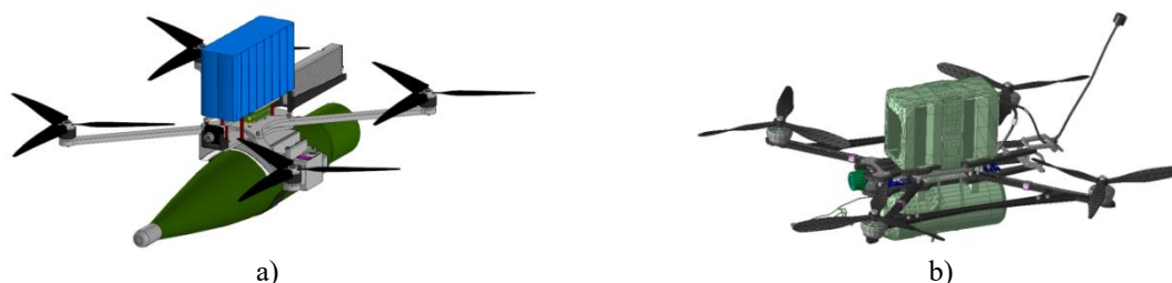
Figure 4. 3D models of FPV drones: a) 10" FPV drone with a payload; b) 7" reconnaissance FPV drone
